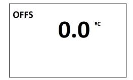
Press  $\checkmark$  **v** to set the sensor in intervals of +-0.5°C, from – 5° C to 5 °C
